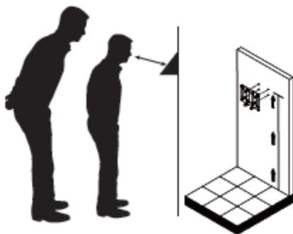
User can drill the holes according to the mounting diagram. Use the 4 wall mount, screws to mount the bracket to the wall. User also could mount the terminal by choosing your “shortest” users and have them stand in front of the device. Hold the terminal on the wall that employee can comfortably center their face in the LCD display window.
